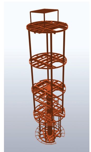
LEFT: Analysis of cantilevered beams and stiffeners on bottom ring to prevent plastic deformation of the central pipe. RIGHT: Raise and Slash Sinking Galloway model.
