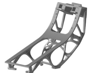
The optimized geometry before and after smoothing.
