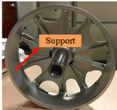
Rotor Hub with Aluminum support
