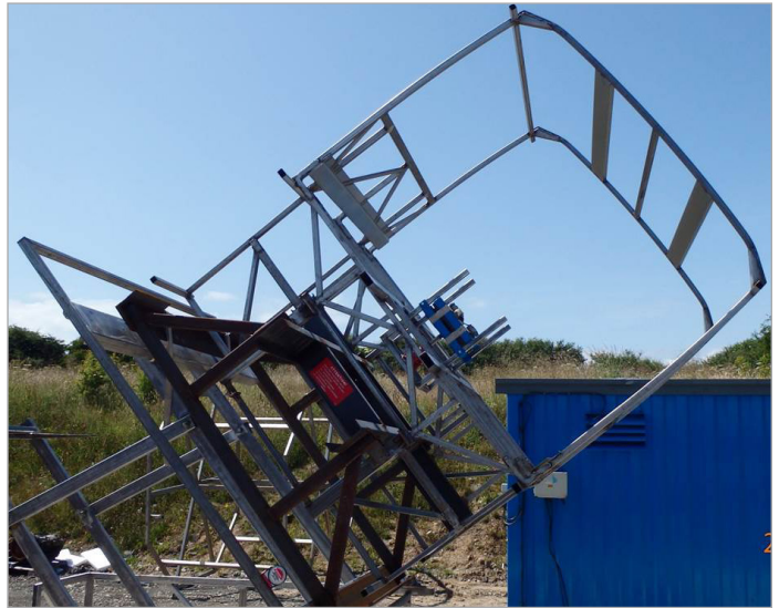
Physical rollover test
