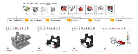
Import and define geometry, create components, set up simulations, and with one-click, analyze and optimize your cast designs.
