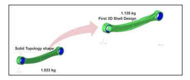
The following table shows the design performance of all load cases after converting the topology geometry to shell mesh model without CAD intervention. Buckling and Durability (stress) being the driving load cases for optimization, the first shell design shows that it is marginally underperforming in Buckling and Durability.
