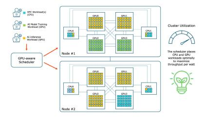
In addition, for partitioned models that span multiple GPU-capable nodes, topologyaware scheduling considers underlying network architectures (where power considerations are also important), including intra-server GPU interconnects and InfiniBand or Ethernet links between servers, minimizing communication overhead and reducing the time and energy required to train a model.
