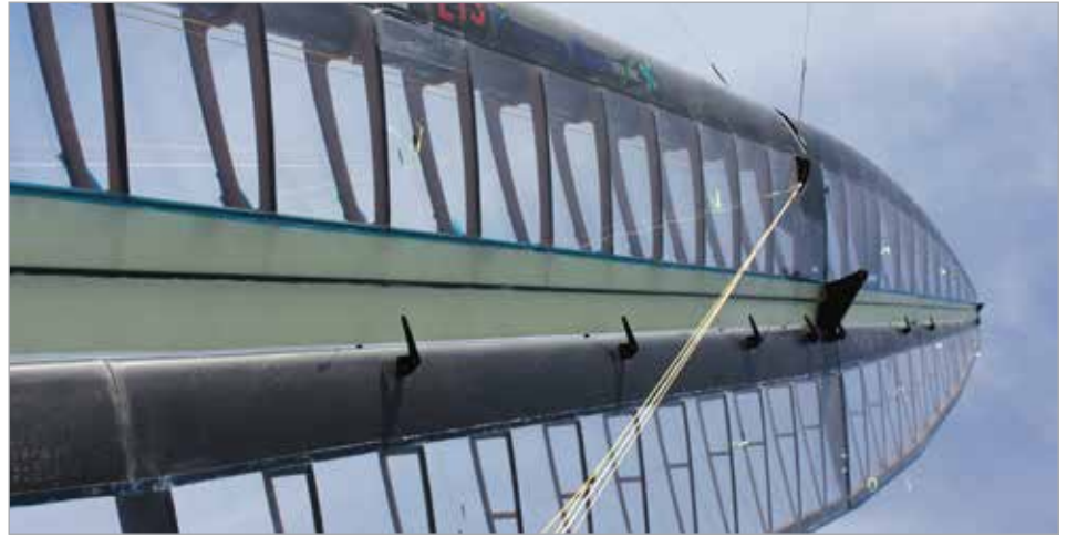
Close-up of the 300 sq ft carbon fiber wing sail
