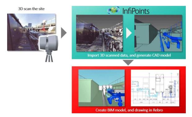
This advanced method, compared to the traditional manual creation of drawings based on on-site measurements, significantly shortens the lead time for BIM model creation, offering a more accurate and time-effective solution for the dynamic demands of equipment and facilities replacement/installation projects.
