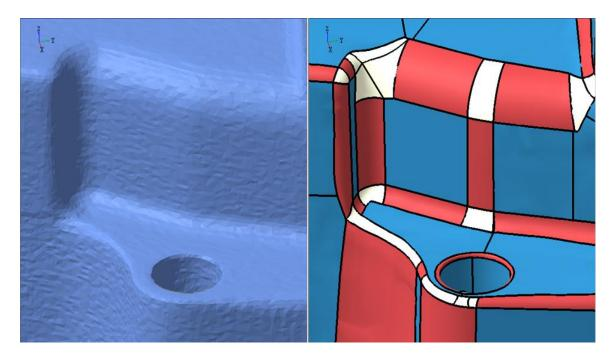
In the realm of CAE, there is a growing demand for quick and straightforward generation of models for simulation. The reverse engineering function of CADdoctor generates Brep models from scanned parts, providing efficient solutions to prepare models for CAE simulation.
