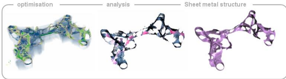
Figure 5: The Optianalyzer Algorithm Generates a Sheet Metal Representation of the Optimum Design.
