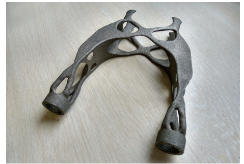
3D Printed Optimized Yoke
