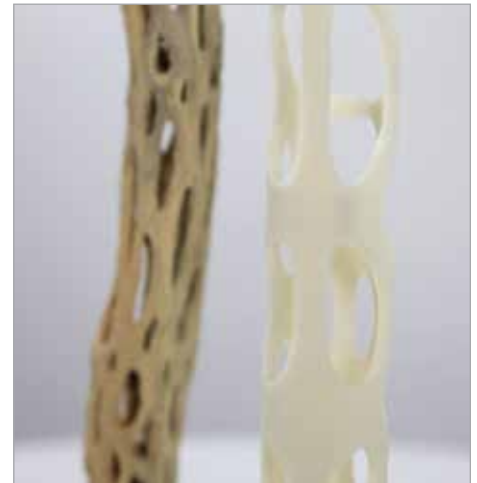
5. The skeleton of a columniform cactus (left) inspired the tubular design of a skyscraper (right).
