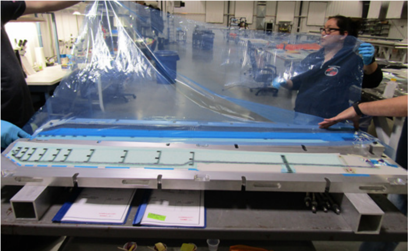
The HVAB blades use Rohacell foam spar cores and pre-cured instrumentation covers and leading-edge skins. ATI bonded the carbon-epoxy HVAB spars and instrumented fiberglass skins. (ATI photo)
