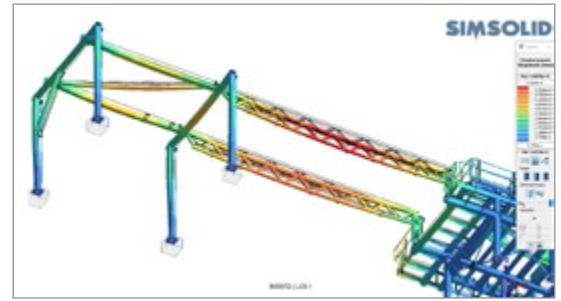
Displacements of the structural frame
