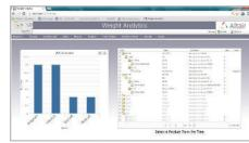
Monitor and analyze KPI's based on Mass, CoG and inertia through a single Web-based interface retrieving information from various company systems
