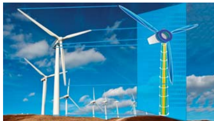
Dynamic digital representations, also called digital twins, use sensor data to mirror a machine in order to understand and optimise its performance, while improving operations
